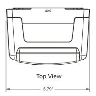
Use the dimensions provided to ensure adequate wall spacing and clearance for the unit.
